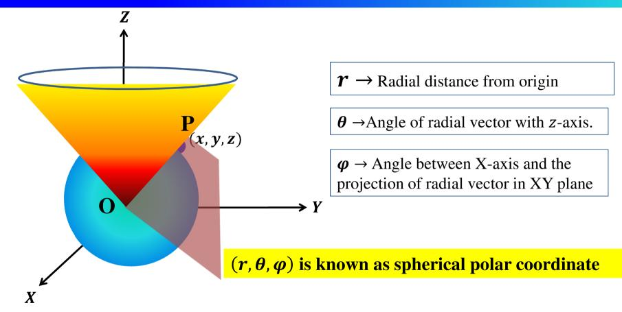
Note that point  $(r, \theta, \varphi)$  is at the intersection of three surfaces
