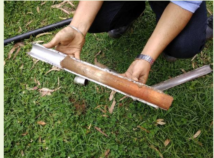
Soil sample collected from SPT
