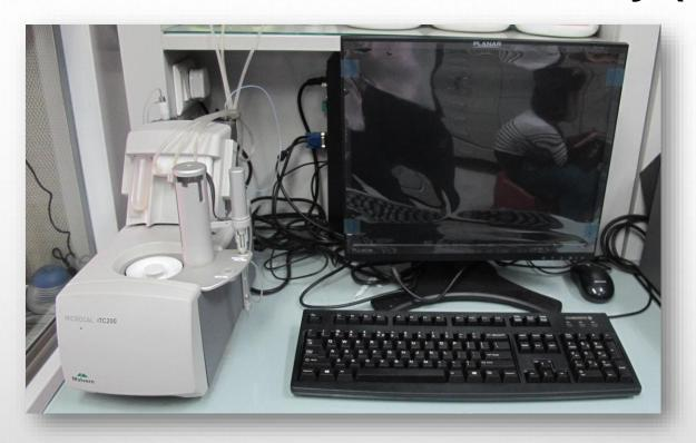
Isothermal Titration Calorimeter (Malvern, MicroCal iTC200) is used to study a wide range of biomolecular interactions. The applications range from drug design to fundamental research. These systems deliver direct, label free and in-solution measurements of binding affinity and thermodynamic parameters.
