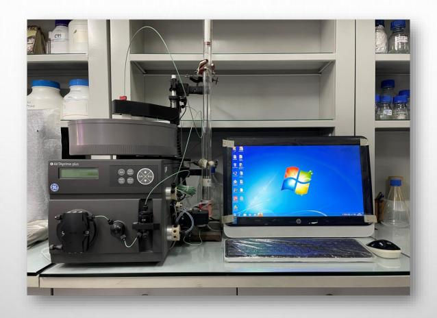
AKTA prime plus chromatography system is a lab-scale protein purification system for purification of biomolecules, providing speed and flexibility in research process.
