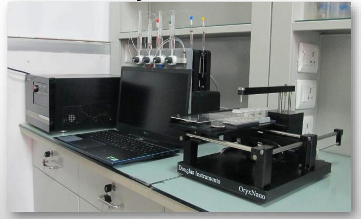
OryxNano, a Protein crystallization Robot for sitting drop method with simple optimization. It is used for large-scale screening of crystallization conditions for proteins.
