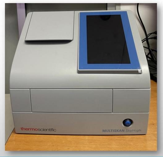
UV-Visible Spectrophotometer (Thermo scientific, Multiskan Skyhigh).
