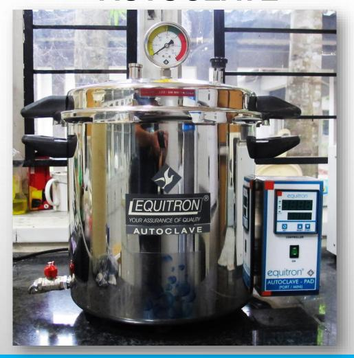
Autoclave system for sterilization.
