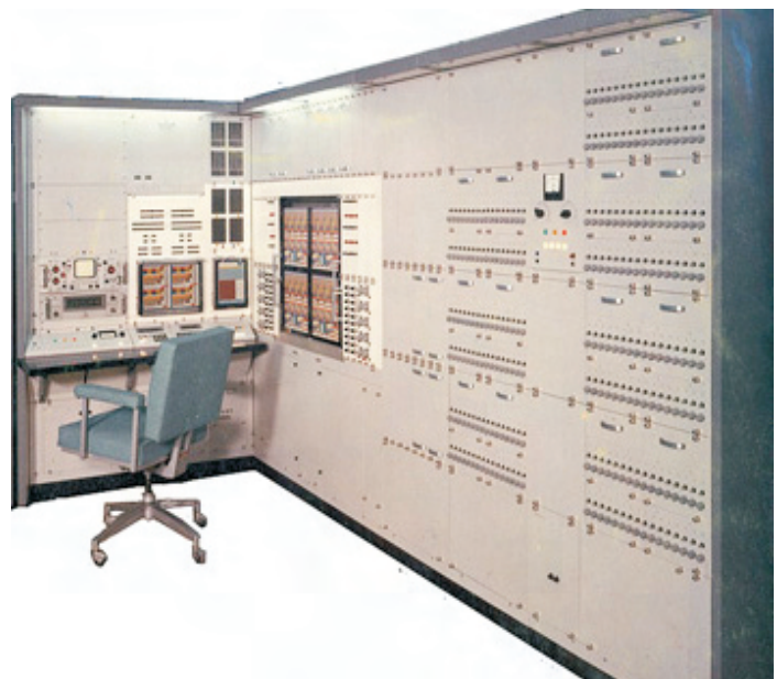
Model AD – 256 released by Applied Dynamics Inc. with 256 amplifiers (Courtesy the Analog Computer Museum and History Center [3])
