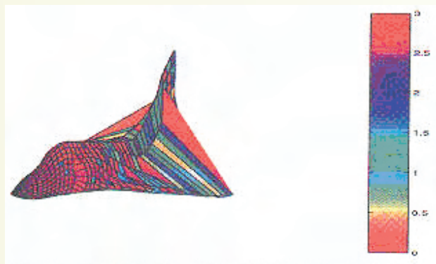
Fig. 3 Current induced on the aircraft by an incident electromagnetic plane wave
