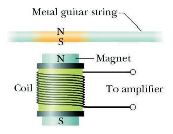
to Pictorial representation of a single coil pickup (only one pole shown) at work
