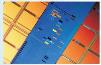
Close-up of a 45nm SRAM Test Wafer
