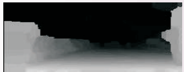
Fig 3. Edge Detection followed by belief-propagation allows to calculate this dense depth map
