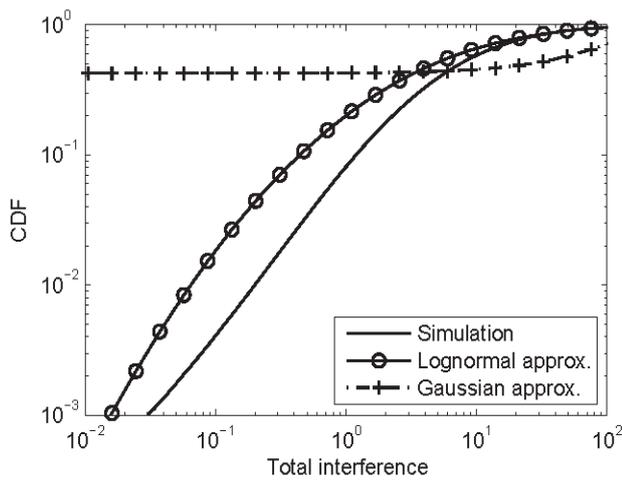
Fig. 2. Comparison of accuracy of CDFs of uplink interference power obtained from the proposed lognormal approximation method and the Gaussian approximation when the average number of users per cell is 10.
