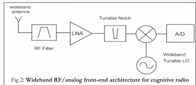
Fig 2: Wideband RF/analog front-end architecture for cognitive radio
