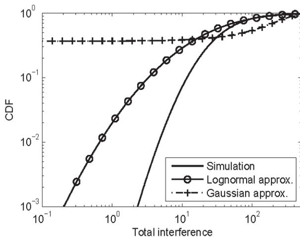
Fig. 3. Comparison of accuracy of CDFs of uplink interference power obtained from the proposed lognormal approximation method and the Gaussian approximation when the average number of users per cell is 30.
