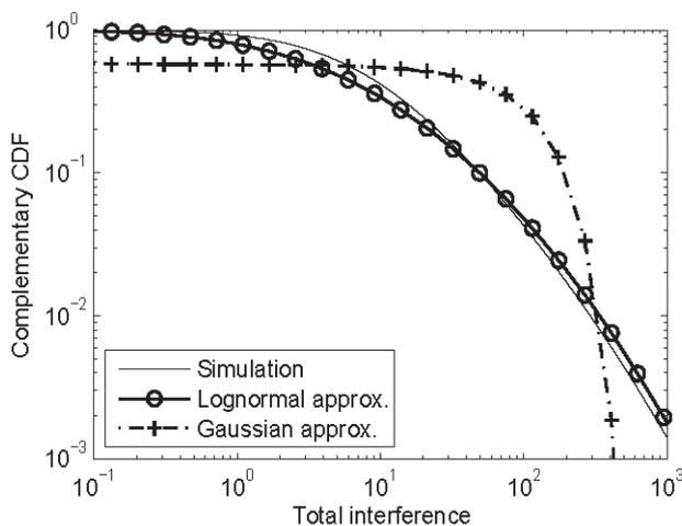
Fig. 4. Comparison of accuracy of CCDFs of uplink interference power obtained from the proposed lognormal approximation method and the Gaussian approximation when the average number of users per cell is 10.
