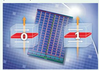
determining the magnitude of tunneling magneto resistance (TMR) in magnetic tunnel junctions (MTJ). Organic spintronics is also a field with upcoming promises. Research in the field of organic spintronics can lead to development in spintronics based organic memories, logic circuits, as well as improve efficiencies of organic light emitting diode (OLED)-based displays.
