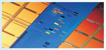
Close-up of a 45nm SRAM Test Wafer
