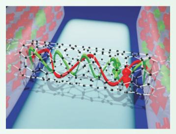
spin space in a spin heterostructure and the application of scheme in spintronic devices. Similar to the Josephson Effect, the equilibrium spin current is generated by the phase difference between the spin wave functions on the two sides of a junction. This problem is of important practical interest, because a spin current can be generated in a spin heterostructure without any external charge current and voltage and the approach has potential applications in low power spintronic devices.
