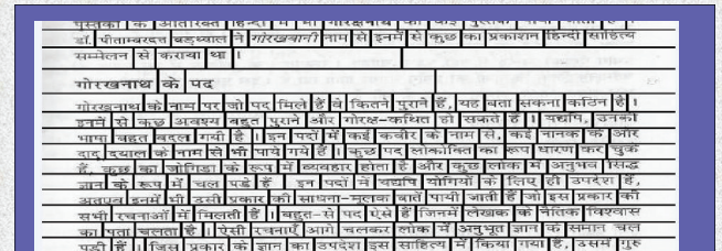
Figure 6: Segmentation of document into set of lines and set of lines into set of words using HPP and VPP.
