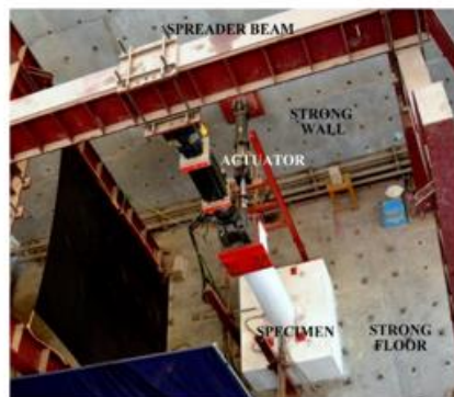
Hybrid testing of bridge pier test model(HyFRC): A bird-eye view
