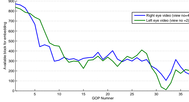
Figure 3.5: Selected blocks for embedding the watermark for each GOP after Z -axis filtration for balloons video ( GOP =8)
