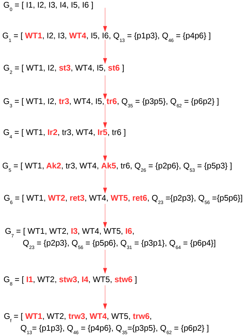
Figure 4.10: Global State Transitions of CFSMs in Fig. 4.9
