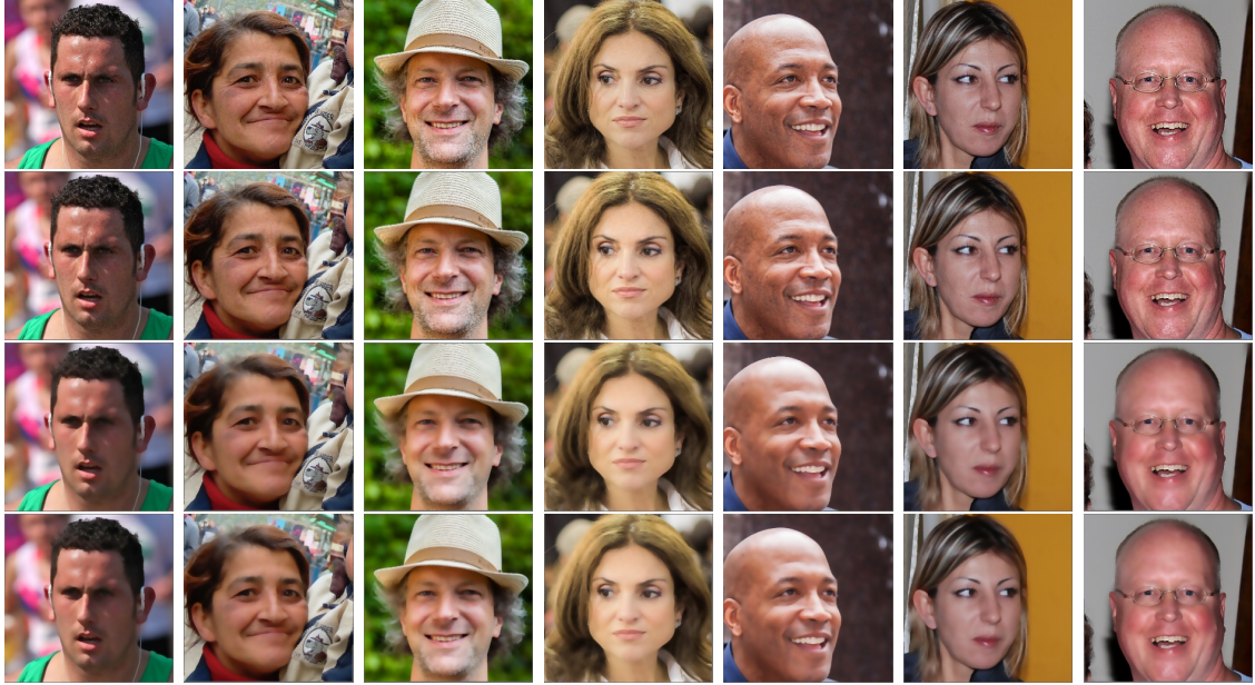
Figure 6.4: Examples of original images, adversarial images generated using FLM, restored adversarial images by BL filter and restored adversarial images by BL+SR (from top to bottom in each column)
