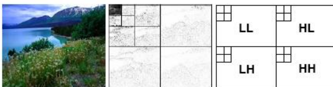
Figure 5.3: The 3-level wavelet transforms for measuring smoothness. The leftmost figure is the original image. The naming convention is shown in the rightmost figure.
