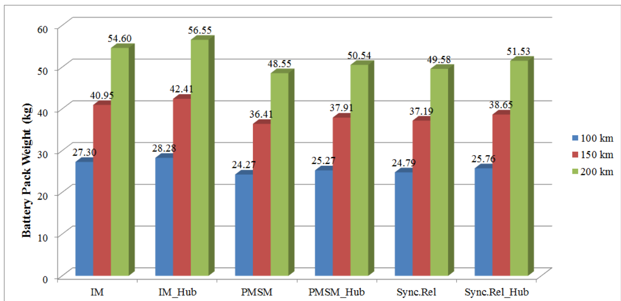
Figure 9.2: Battery pack weight (in kg) for various motor configurations at different range requirements - Honda CB Shine 125 cc
