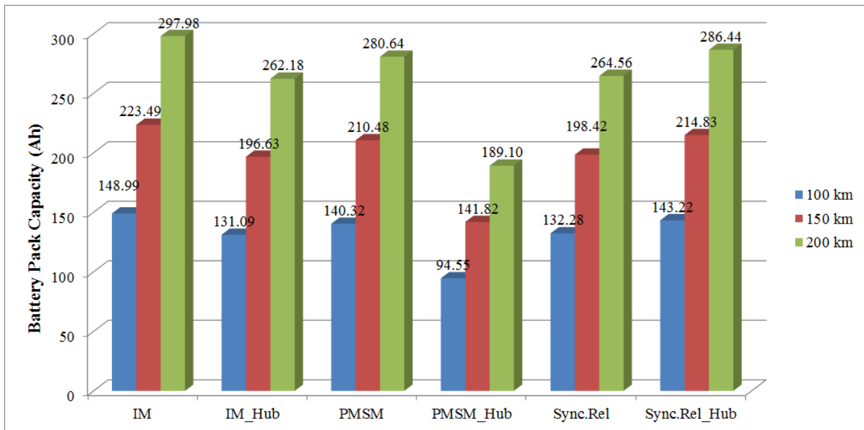
Figure 9.11: Battery pack capacity (in Ah) for various motor configurations at different range requirements - Retro bike
