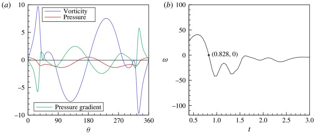
FIGURE 17. (a) Distribution of vorticity  $\omega$ , pressure  $p$  and the pressure gradient  $p_\theta$  along the surface of the cylinder at the time of the second structural bifurcation  $t = 0.828$  and (b) time history of vorticity at the point  $\theta = 44.8^\circ$  on the cylinder surface.
