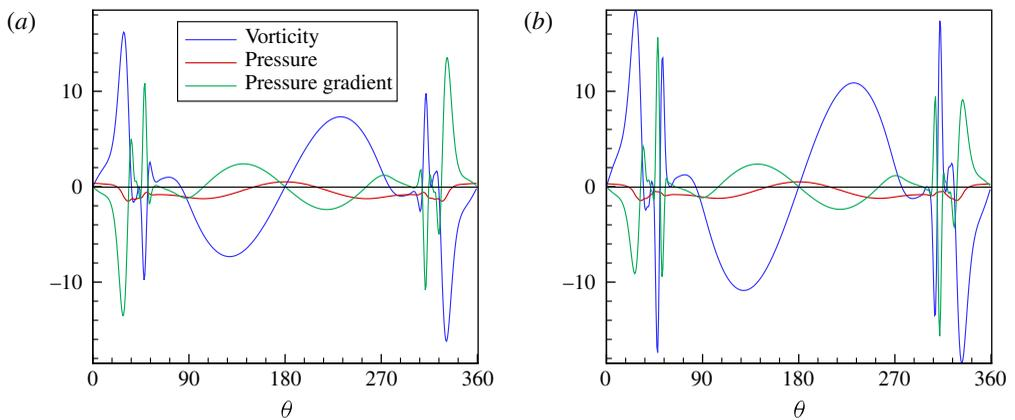
FIGURE 22. Distribution of vorticity  $\omega$ , pressure  $p$  and the pressure gradient  $p_\theta$  along the surface of the cylinder at the time of the formation of the tertiary vortices: (a)  $t = 1.116$  and (b)  $t = 1.233$ .
