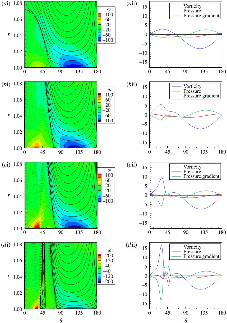
FIGURE 20. Combined streamfunction and vorticity contours (column i) and distribution of vorticity  $\omega$ , pressure  $p$  and the pressure gradient  $p_\theta$  along the surface of the cylinder (column ii) at times (a)  $t = 0.45$ , (b)  $t = 0.70$ , (c)  $t = 0.80$  and (d)  $t = 1.0$ . Note that the streamlines are plotted using lines, with the dotted lines representing negative contour values, and the colour scale is used for plotting the vorticity contours.
