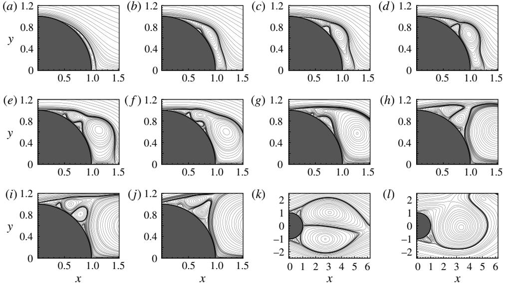
FIGURE 6. Evolution of streamlines for  $Re = 5000$  for flow past a circular cylinder at: (a)  $t = 0.5$ , (b) 0.9, (c) 1.0, (d) 1.1, (e) 1.35, (f) 1.45, (g) 1.7, (h) 2.25, (i) 2.9, (j) 4.0, (k) 20.0 and (l) 24.5.
