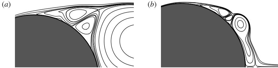
FIGURE 1. (a) The  $\alpha$ -phenomenon (for  $Re = 3000$  at time  $t = 2.5$ ) and (b) the  $\beta$ -phenomenon ( $Re = 9500$  at time  $t = 1.0$ ): the streamlines are generated from our own computation.
