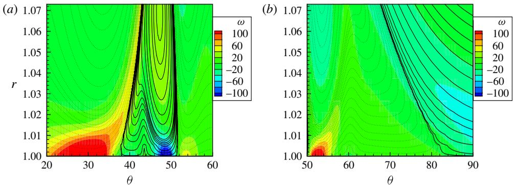
FIGURE 24. Combined streamfunction and vorticity contours showing spike formation before the separation leading to the tertiary vortices: (a)  $t = 1.115$  at  $\theta = 43.2^\circ$  and (b)  $t = 1.23$  at  $\theta = 60^\circ$ .
