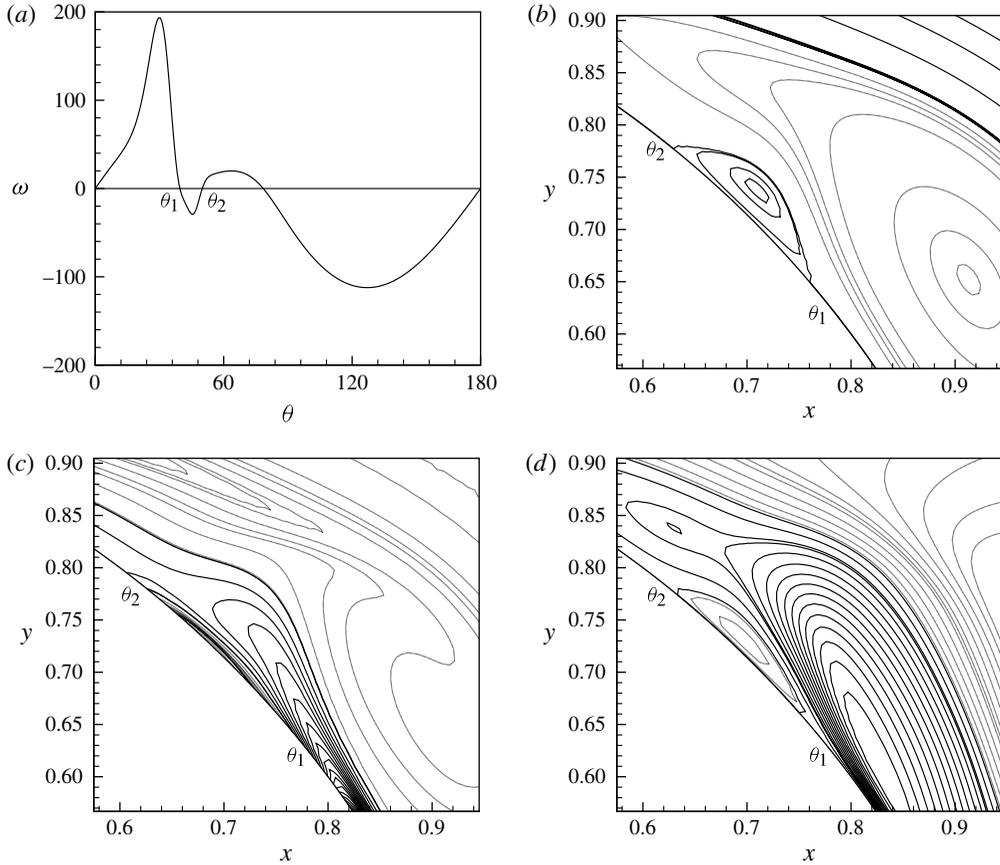
FIGURE 18. At time  $t = 0.90$ : (a) vorticity distribution on the surface of the cylinder, (b) streamfunction contours, (c) vorticity contours and (d) vertical velocity contours. In (b–d), the dotted lines denote contours with negative values.
