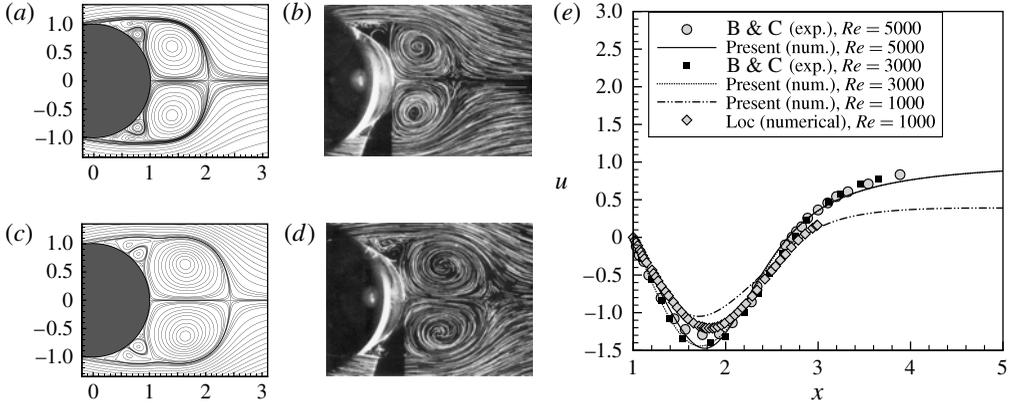
FIGURE 2. Comparison of streamlines with experimental results of Bouard & Coutanceau (1980)(C & B) for  $Re = 5000$ : (a) present ( $t = 2.0$ ), (b) experimental ( $t = 2.0$ ), (c) present ( $t = 2.5$ ) and (d) experimental ( $t = 2.5$ ); and (e) comparison of velocity distribution on the flow axis between experimental (Bouard & Coutanceau 1980), numerical (Loc 1980) and the present results at  $t = 3.0$  for  $Re = 1000, 3000$  and  $5000$ .
