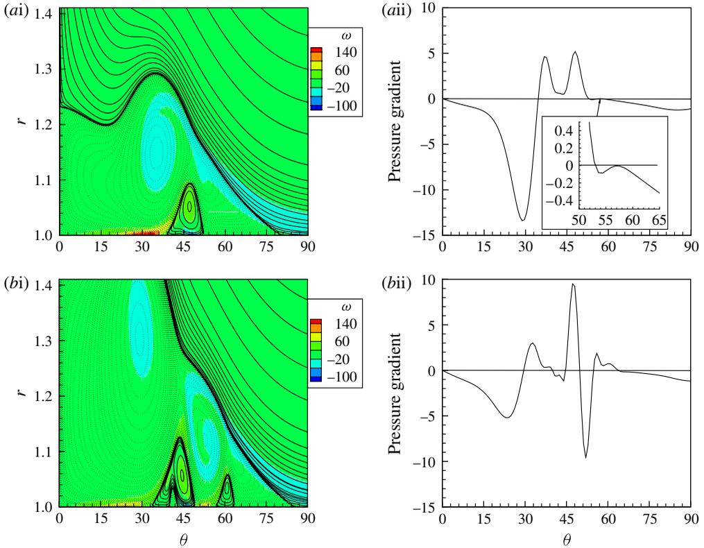
FIGURE 21. Combined streamfunction and vorticity contours (column i) and distribution of pressure gradient  $p_\theta$  along the surface of the cylinder (column ii) at times (a)  $t = 1.0$  and (b)  $t = 1.35$ .
