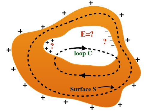
There can not be any field inside a cavity within a conductor, nor any charges on the inside surface.
