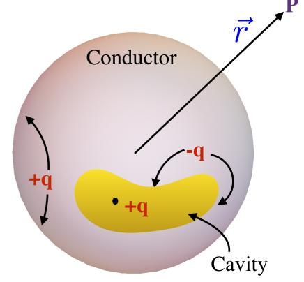
The charge +q induces an opposite charge -q on the wall of the cavity, which distributes in such a way that its field cancels that of +q, for all points exterior to cavity.
