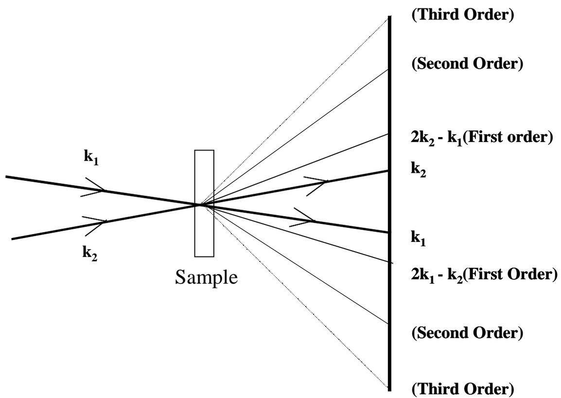
**Fig. 2.7** Experimental setup for the Forward Four Wave Mixing
