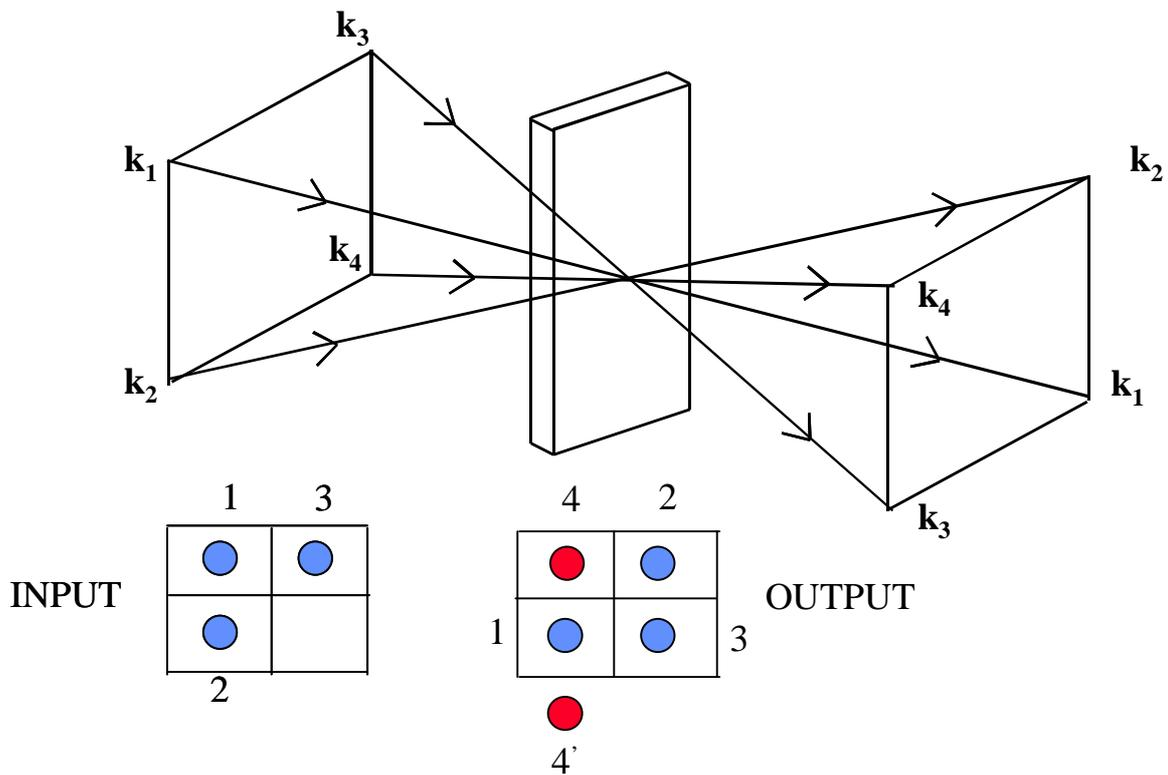
**Fig. 2.6** DFWM set-up in the boxcar configuration. 4 and 4' are the signals
