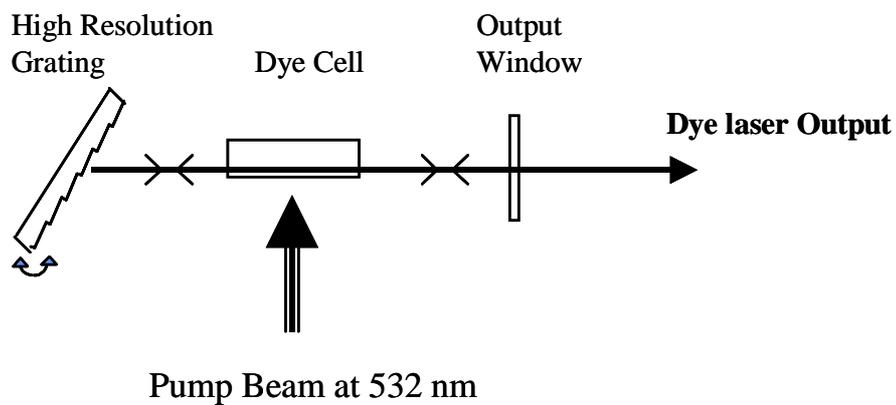
**Fig. 2.2** Home built dye laser with (a) Mirror and (b) Grating as tuning elements.
