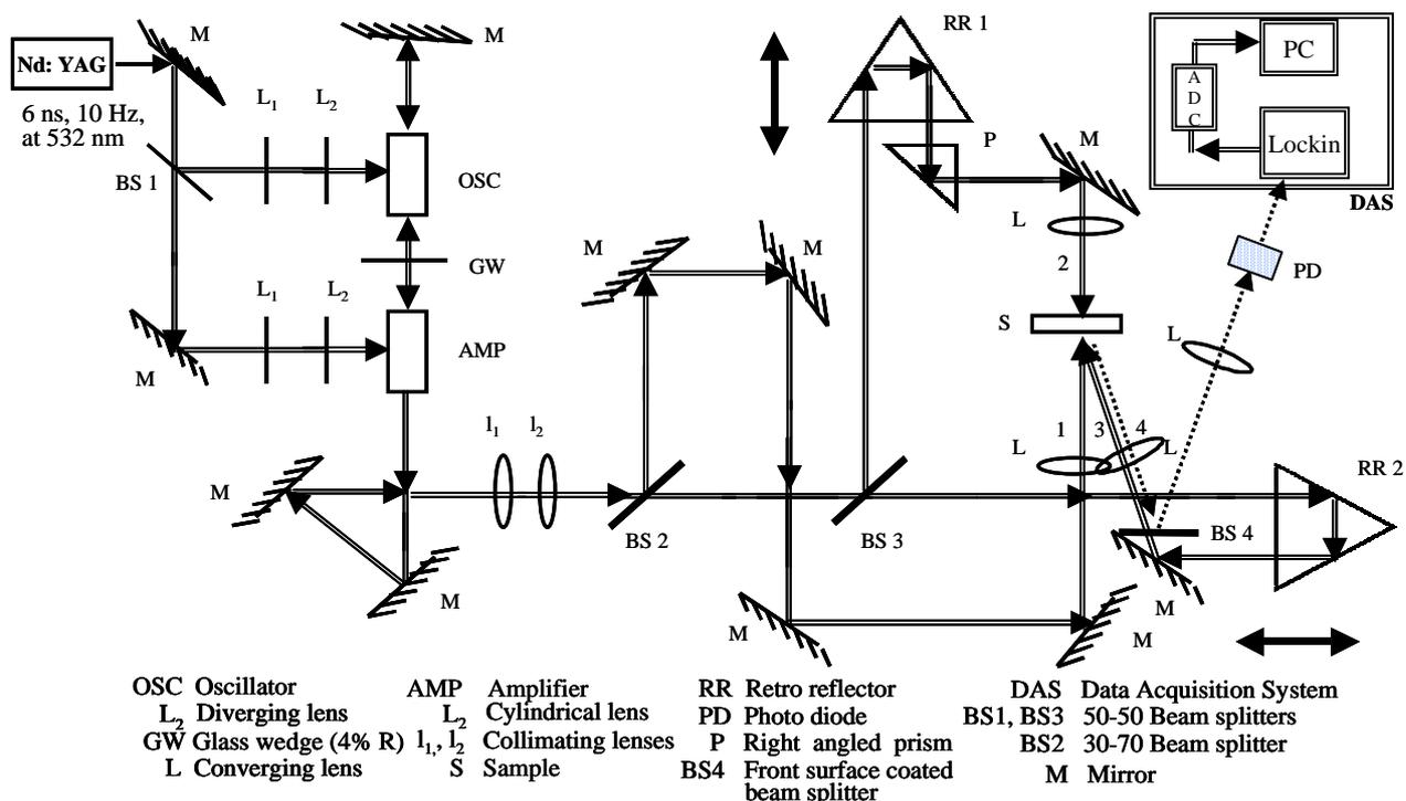
**Fig. 2.5** Experimental setup for Degenerate Four Wave Mixing with Incoherent Light
